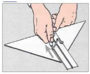
3.2.3 The filler is cut to the required height of the skirting.
