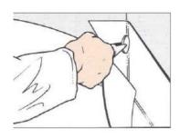
3.1.3 Cut the excess material to the 45 degree angle.
