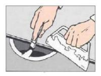
Heat the floor covering gently and fit it into the floor drain. Fit the clamping ring and double check the adhesion for water tightness. The edge of the installed floor covering should then be sealed.
